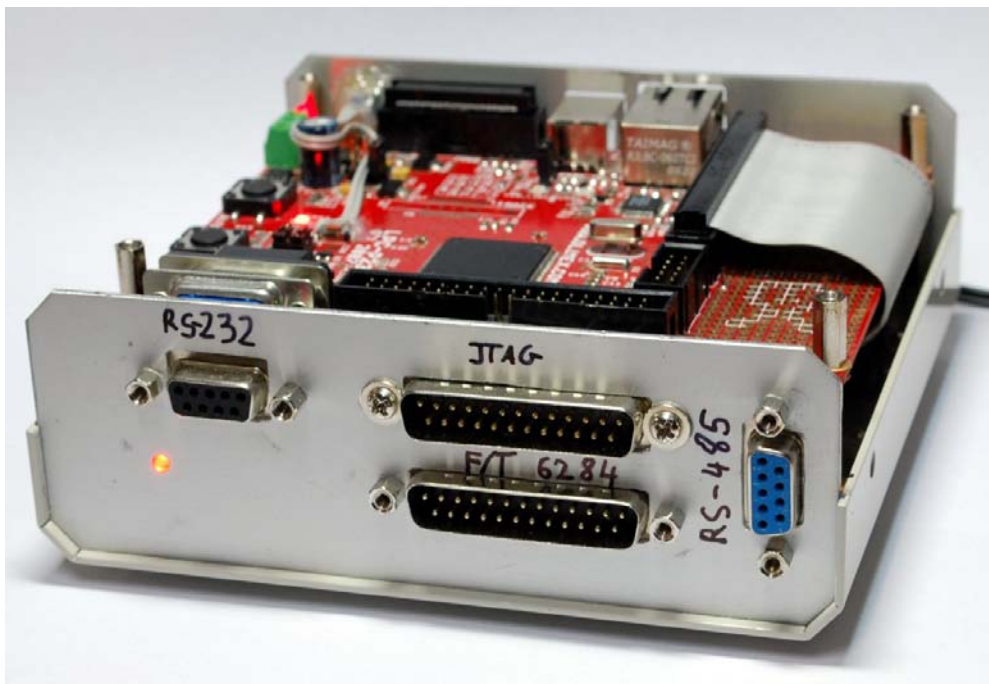
Figure 5.1. Force/torque sensor controller
